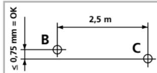
**!** Regularly check the adjustment before use, after transport and after extended periods of storage.
